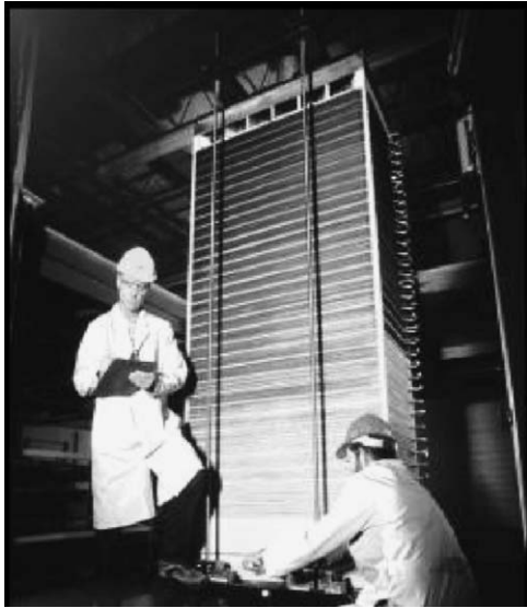
Fig. 1. Full-size stack completed at the FCE manufacturing facility: ~350–400 cell stack.
