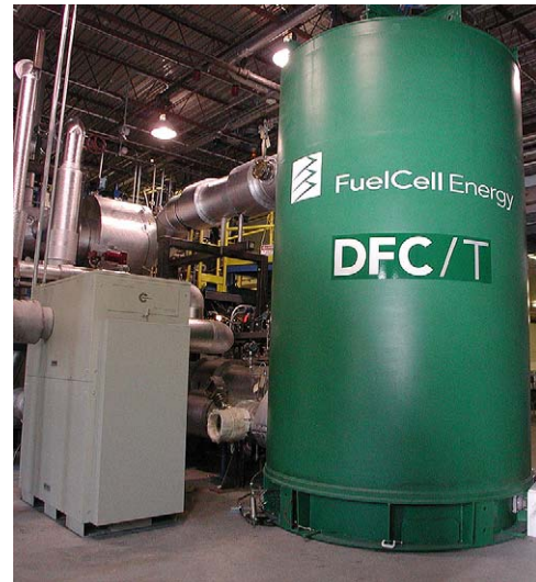
Fig. 4. Direct FuelCell/turbine hybrid system.
